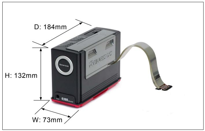
Figure 7.2 External dimensions of the E100 emulator
